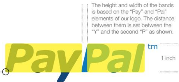
The minimum size of the twin bands is determined by the height, which may not be less than 0.25 inches and the minimum size of the radii may not be less than 2pt.
